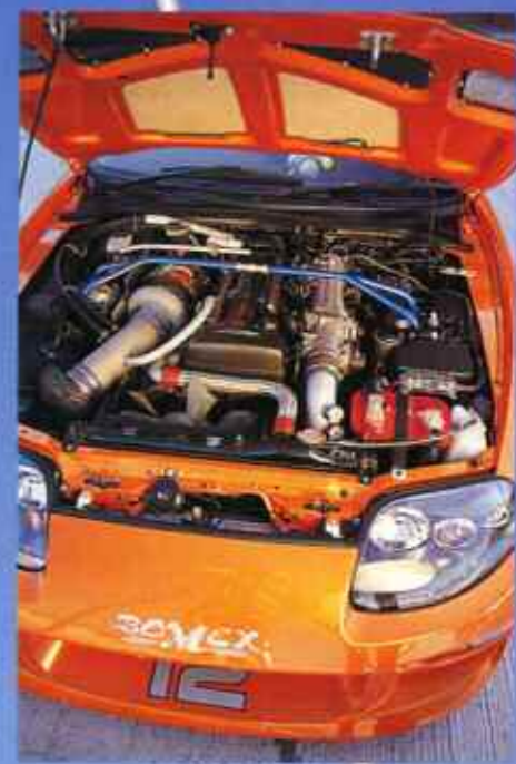
Supra's 3-litre six has had the twin-turbo system ditched in favour of a massive GReddy single T88 unit with HKS intercooler, 650cc injectors and Blitz electronics
